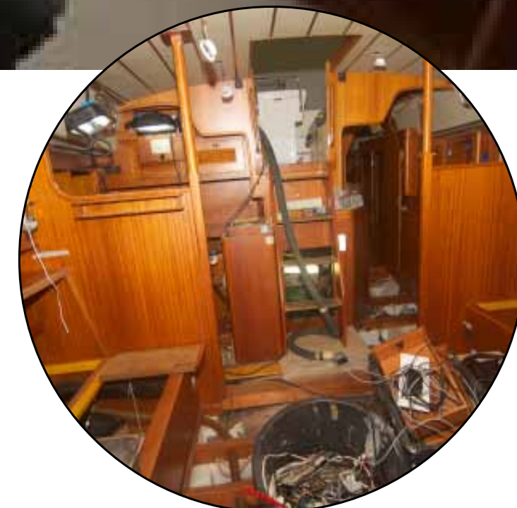
▲ Above: the boat's interior was almost completely dismantled so that everything visible and out of sight could be refurbished or replaced. The work was done in an ad hoc yard Schulz set-up in Sweden that used former boatbuilders from some of the best-known Swedish production builders
