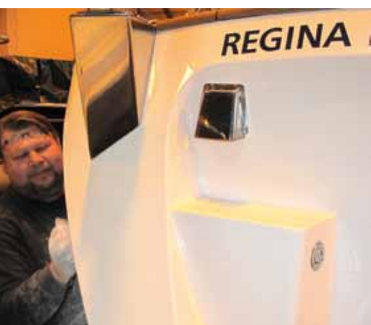
◀ Left: the condition of the stern was particularly poor which entailed removing and refitting everything including backstay chainplates. Above: it took 60 hours to re-polish the topsides. Right: re-varnishing and new lighting completely changed the ambience of the HR46's saloon.
