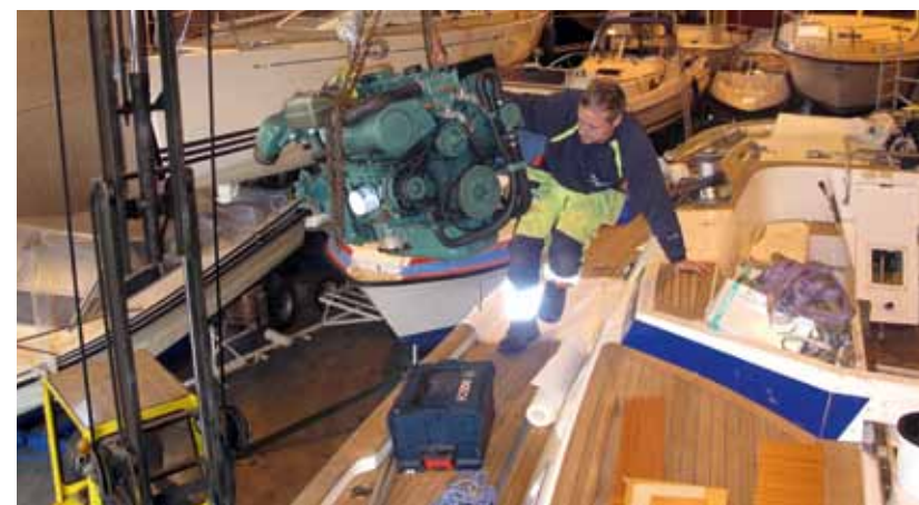
The original Volvo TMD31 engine was overhauled but most of its ancillary equipment was replaced. Below: the engine is removed.
