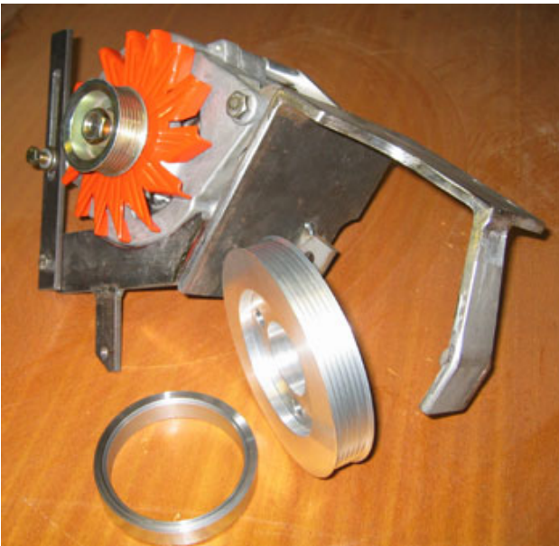
The first pictures of the AMPTECH 160A on the brackets for the Volvo D2-55 together with the new pulley. The V-belt is a standard Volvo belt, part No 3581460
