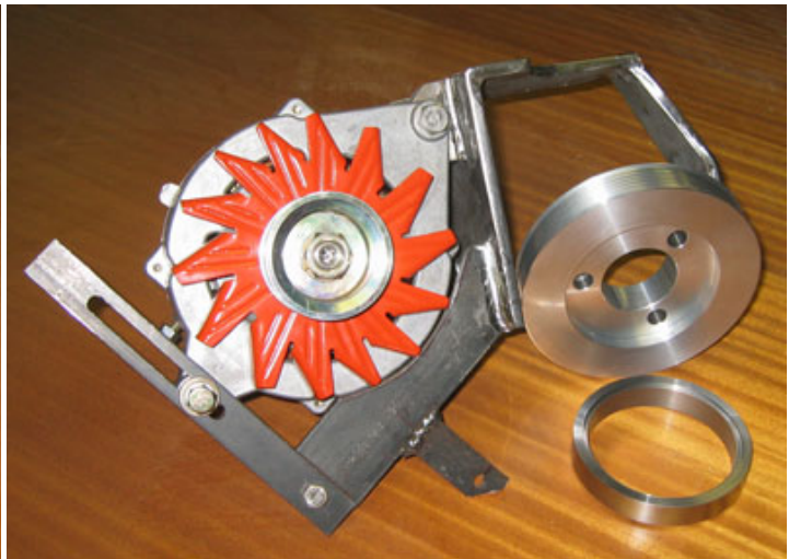
The first pictures of the AMPTECH 160A on the brackets for the Volvo D2-55 together with the new pulley. The V-belt is a standard Volvo belt, part No 3581460
