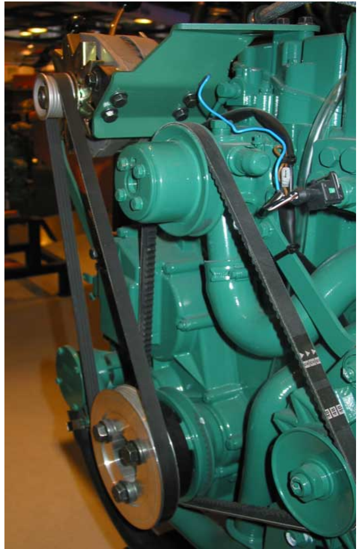
Volvo's own 220V system installed on a D2-55 engine shown at an exhibition.
