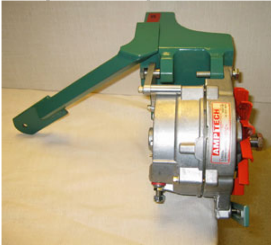
The new amended brackets with an arm showing aft instead of to port now fixed with "Screw B"
