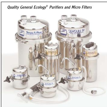
SEAGULL IV water purifier operates at a minimum water pressure of about 25 psi. General Ecology offers manual pumping purifiers for systems having inadequate pressure. Systems with both one and two GPM flow rates are available.
