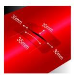
If you are repairing a tear or rip that is longer than 35mm in any direction you will need to apply an inside patch. If the hole is less than 35mm you can apply
