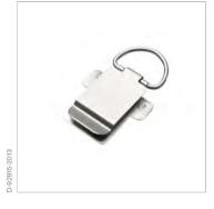
The belt clip can be used with any standard belt. Ideal for short term applications like inspection or maintenance where the unit is often attached to and removed from the belt. Can be mounted on the Hard Case using the accessory attachment points. For attachment on the Soft Pack the adapter plate is needed. (Order number: R 59 456)
