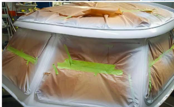
Above left: prep work for the Coppercoat. Above: finished Coppercoat on hull and Propspeed on the propeller. Left/right: hardtop repainted and all windows replaced with new aluminium frames, handmade by the same person who originally made them in 1996.
