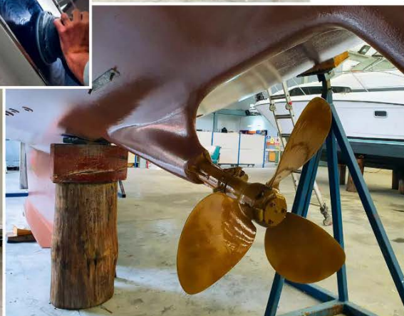
Above left: prep work for the Coppercoat. Above: finished Coppercoat on hull and Propspeed on the propeller. Left/right: hardtop repainted and all windows replaced with new aluminium frames, handmade by the same person who originally made them in 1996.
