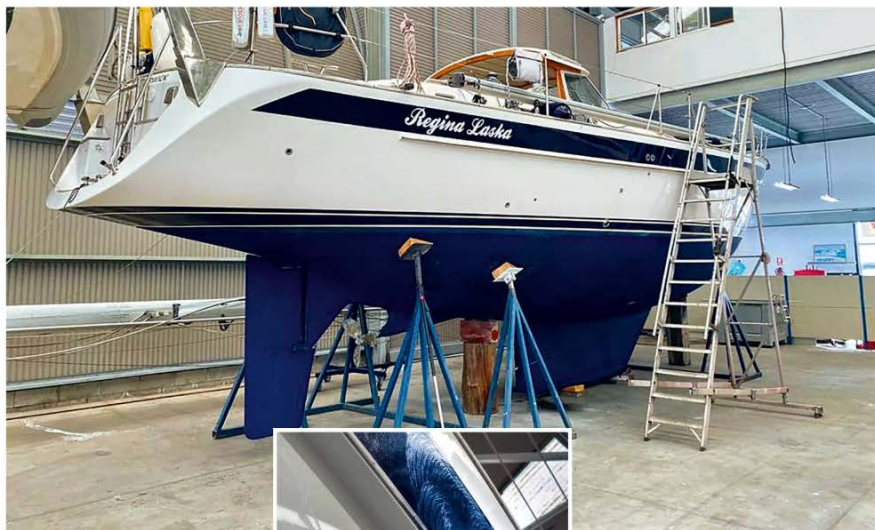
Left: preparing to strip off the antifouling and epoxy a second time after 2013. Inset: annually polishing the repainted famous HR blue stripes.
