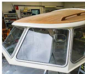
Above left: prep work for the Coppercoat. Above: finished Coppercoat on hull and Propspeed on the propeller. Left/right: hardtop repainted and all windows replaced with new aluminium frames, handmade by the same person who originally made them in 1996.
