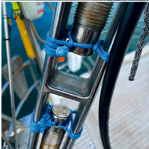
Above: turnbuckles were changed after 25 years.
