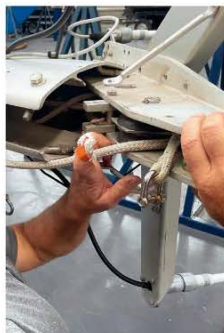
Above: turnbuckles were changed after 25 years.
